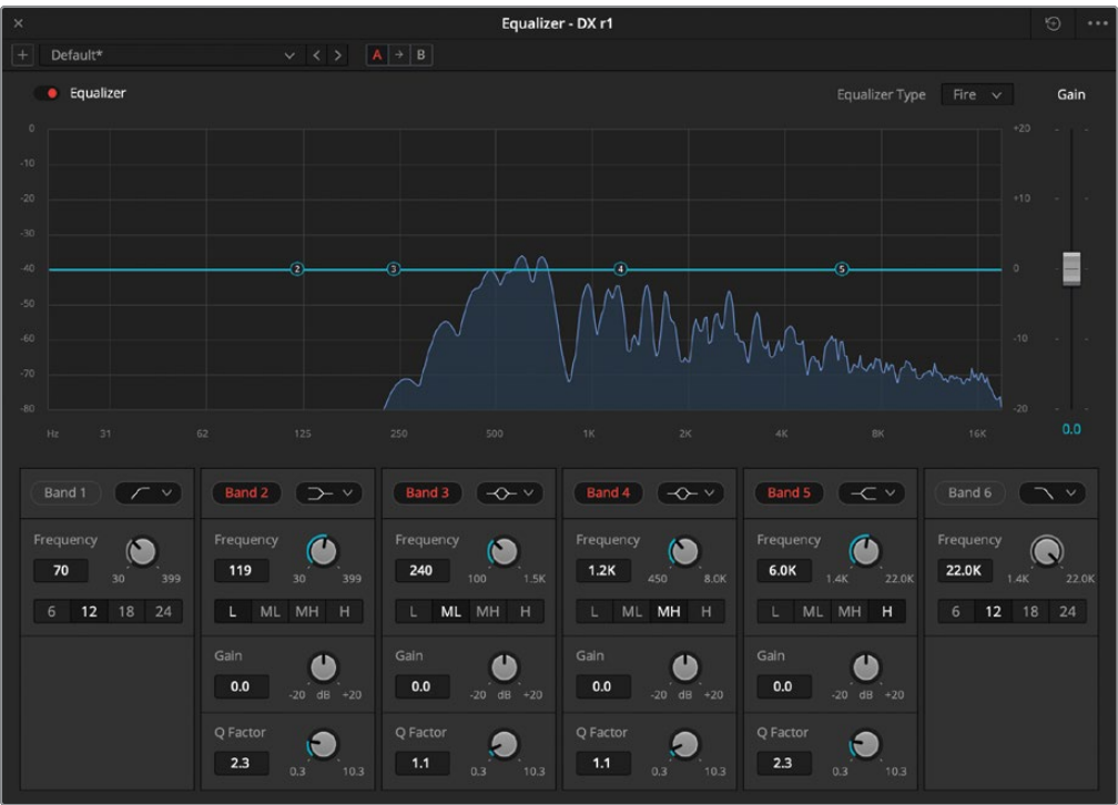
Fairlight Track EQ window showing real-time dialogue frequencies during playback
